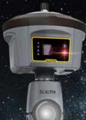
SOUTH brand-new image RTK V1 surveying system consists of Galaxy G6 and image acquisition system which combined with new point positioning technology--Touch. It crosses space obstacles and sweeps measurement blind area by taking three pictures to obtain the target coordinate information.(unreached points with ordinary RTK system)
