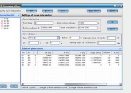
2) Enable to calculate and display track gauge, horizontal, triangle pit, 30m chord left and right orbit, 30m chord left and right height; adopt Track Quality Index (TQI) calculation and evaluation, apply to 50-200 m section, and adjust the poor ride performance of track long-distance section;
