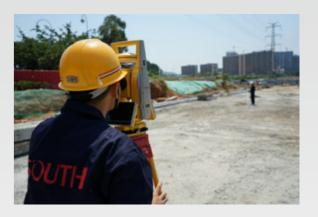
Mission: Plan to stake-out the position of buildings, facilities or roads on the site. Due to the limitation of working environment and the obstacle, most of them are unable to set a RTK rover stably,
