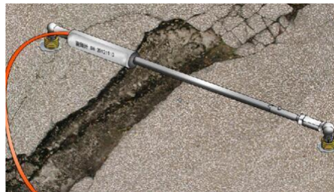
Vibrating wire crack gauge
