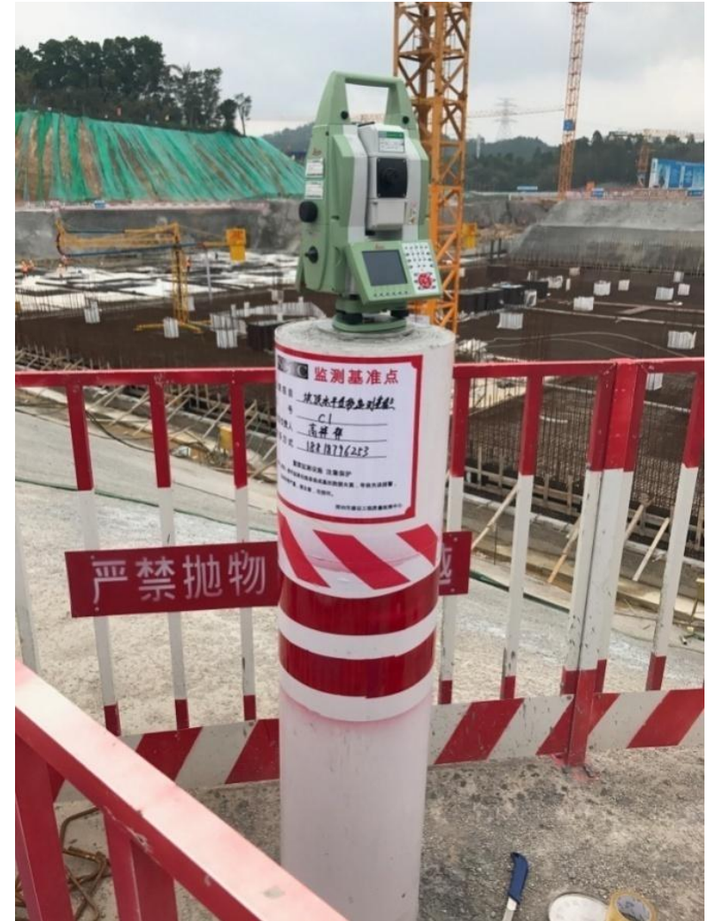
Robotic total station with APP and prisms
