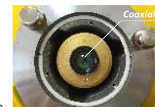
Coaxial Design of Tx/Rx Unit
