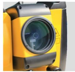
> 600m reflectorless measurement
