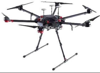
Option 1: DJI Matrice 600 Pro (to fit LiDAR-eco Pro + camera)
