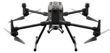
Option 3: DJI Matrice 300 RTK (to fit LiDAR-eco Pro only)
