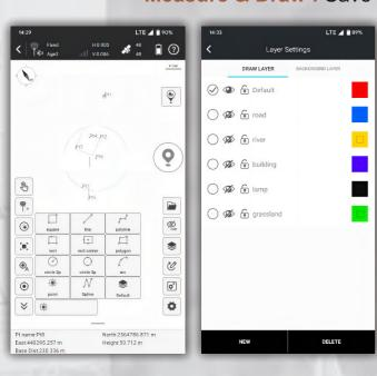
This feature allows you to draw the result map while completing point measurements.
