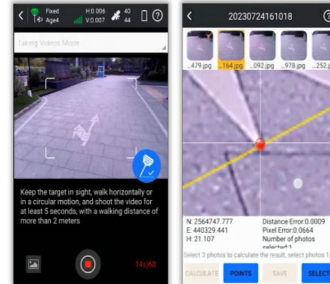
Photogrammetry Measurements can be conducted by taking pictures or videos. Coordinates of all points in the photos can be acquired.
