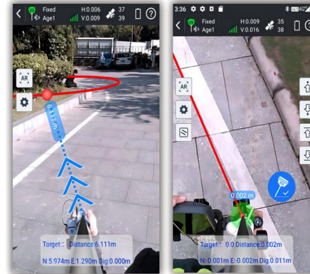
Users utilize the real-time imagery captured by the camera at the bottom of the receiver and the AR guide lines displayed by the software, to locate the target points.
