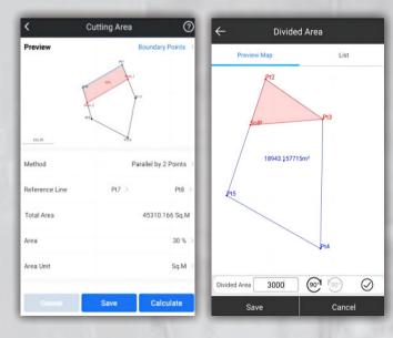
Select points to form a polygon, and directly identify the area division points for the surveyor to stake out. There is no more need for the user to guess a position to measure, and then to adjust.
