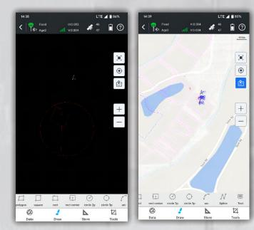
Select points to form a polygon, and directly identify the area division points for the surveyor to stake out. There is no more need for the user to guess a position to measure, and then to adjust.
