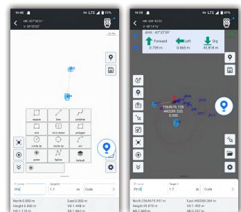
The App Now works with GNSS, Total Station, Echo Sounder, GIS Tablet, in future it will work with SLAM Scanner, Terrestrial Lidar Scanner.
