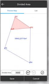
Select points to form a polygon, and directly identify the area division points for the surveyor to stake out. There is no more need for the user to guess a position to measure, and then to adjust.
