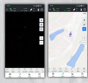
Select points to form a polygon, and directly identify the area division points for the surveyor to stake out. There is no more need for the user to guess a position to measure, and then to adjust.
