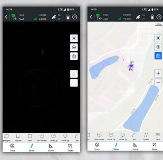
Select points to form a polygon, and directly identify the area division points for the surveyor to stake out. There is no more need for the user to guess a position to measure, and then to adjust.
