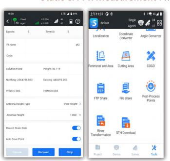
The software provides both static and PPK data collection capabilities.
