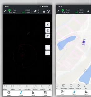
Select points to form a polygon, and directly identify the area division points for the surveyor to stake out. There is no more need for the user to guess a position to measure, and then to adjust.
