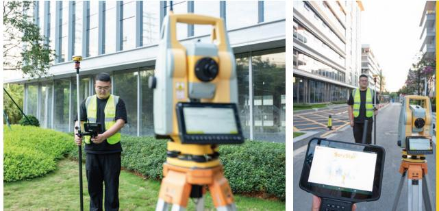
The ZigBee module enables connection to robotic total stations, either alone or in conjunction with GNSS receivers, allowing for faster prism tracking and expanding your work scenarios. On H7, you will have a full and larger screen to fulfill your daily CAD
